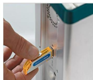
The DataLogger function copies all measurement series directly on to a USAB stick.
